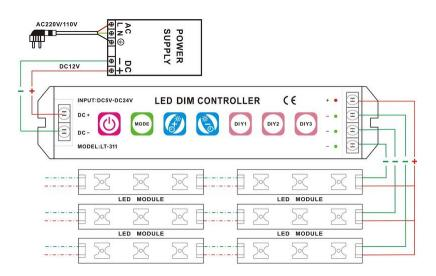
Collect to single color high power LED lamps, the controller provides controlling signals only; the lights need extra power based on the specific working voltage of the lights. Each controller theoretically can control unlimited quantity of the lamps.
