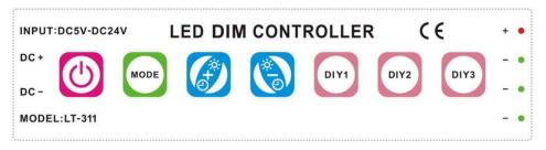
The controller has 7 function keys:
