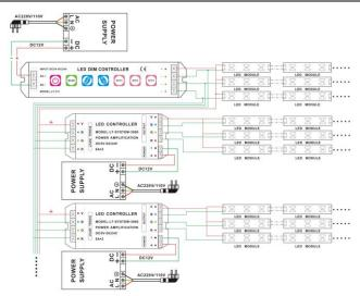
Method Two: Connect the controller and the amplifier by a method of "hand in hand".
