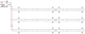
! 30 pcs - max number of modules in one chain when the power supplied from single end. ! String end voltage can't be less than 11V, do not exceed specified module string length.
